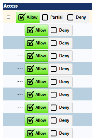
Figure 9.9. The "allow" status assigned to the main menu cascades to all of its submenus.
